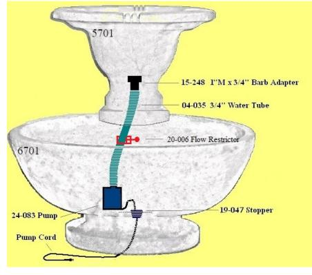
5) Thread the 15-248 1" male x <sup>3</sup>/<sub>4</sub>" barb adapter into the underside of the 5701 top unit.
