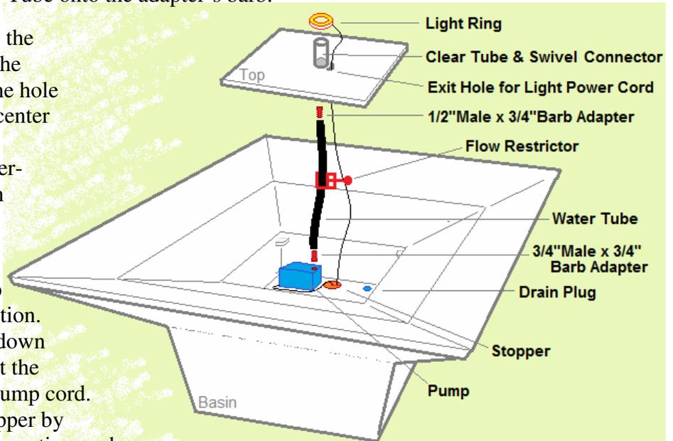
5) Place the Flow Restrictor in the middle of the water tube. Tighten it just enough to hold in place on the tube. (Later, if you want to turn down the amount of water flow in your fountain, you can tighten this further to make that adjustment.) Push the open end of the water tube over the barbed adapter underneath the fountain top. Then set the fountain top down on the ledges inside the basin. Make sure it is centered.
