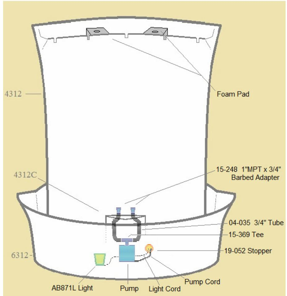
6) Thread the tee into the top of the pump. Then attach the open ends of the tubes to the tee barbs. Set the 4312C pump cover in front of the pump area to hide the pump and tube connection.
